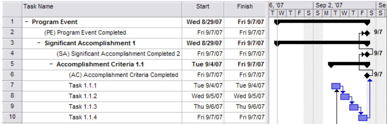
Figure 9 – The connections of tasks within the AC must land on the place holder for the AC. Because Microsoft Project does not allow linkage to Summary Tasks (Primavera calls these hammock task), an ersatz task is needed to “hold the place” of the AC. The same is the case for the SA and PE. With these place holders and complete “network” can be constructed for the IMS and IMP. No widows or orphans for any element.
